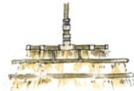
SPRAY BAR FOR DUST CONTROL
